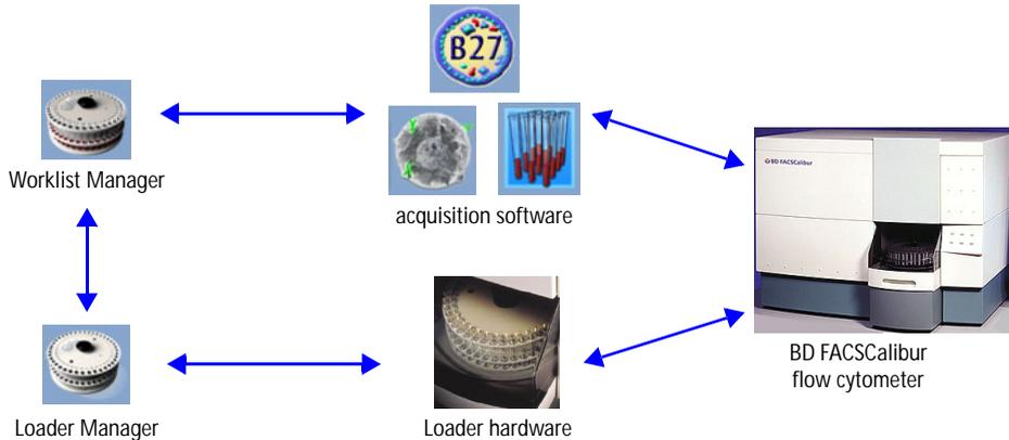
When Worklist Manager is launched, it automatically launches Loader Manager and verifies the Loader is connected. The Worklist Manager application window and the Loader Manager Status window appear on the desktop.
