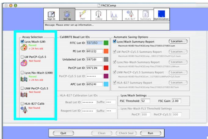
For lyse/wash (LW) or lyse/no-wash (LNW) assays, the software automatically performs 2-, 3-, or 4-color setup based on the BD Calibrite bead lot IDs and the bead populations detected.
