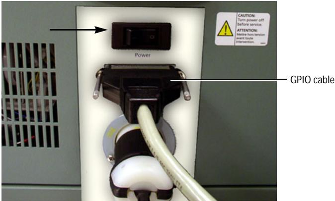
**Figure 1-11** Transformer main power switch (230 VAC)
